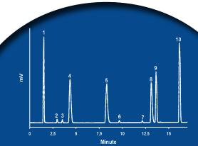
Multimodal stationary phase HPLC/ELSD chromatogram of the simultaneous analysis of polar and non-polar, neutral, acidic and basic pharmaceutical drugs and their counterions
